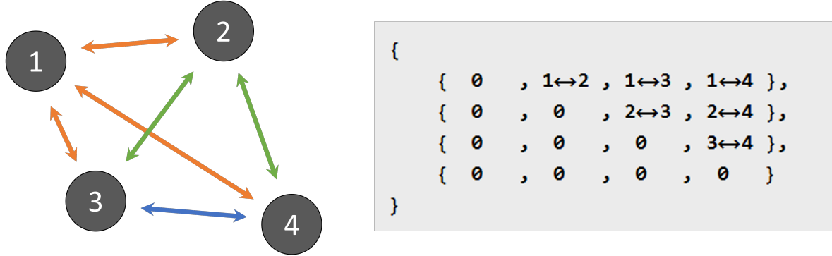
Figure 5.12.: Example of four molecules with the corresponding interactions between them (arrows) on the left side and the structure of the array containing the energy information of those interactions on the right side.
